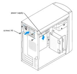
6. Remove the power supply from the computer.
