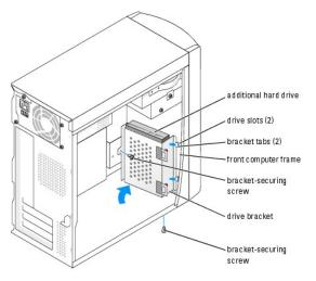
8. <u>Reinstall the existing hard drive</u> into the computer in front of the additional drive.
