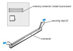
4. Align the notch on the bottom of the module with the crossbar in the connector.
