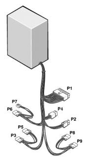
The 305-W power supply can operate from an AC power source of 115 VAC or 230 VAC at 50 - 60 Hz. The power supply provides the DC operating voltages and currents listed in the following table.
