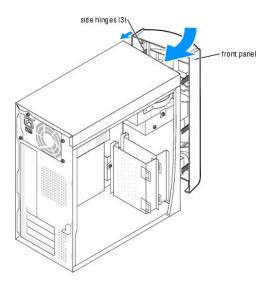
2. Rotate the front panel until it snaps onto the front of the computer.
