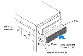
4. After the drive is in place, apply pressure to ensure that the drive is fully seated.
