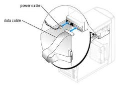
S NOTICE: Match the colored stripe on the cable with pin 1 on the drive (pin 1 is marked as "1").
