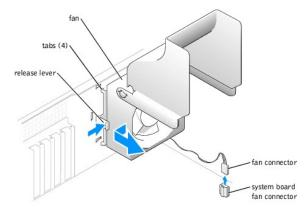
7. Remove the fan assembly from the computer.
