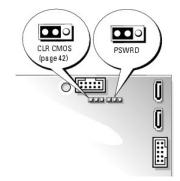
2. Locate the 3-pin password jumper (PSWD) on the system board, and attach the jumper plug to pins 2 and 3 to clear the password.
