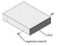
NOTE: Some computers come with only two extra alignment screws; others come with four. You only need two alignment screws for this procedure.
