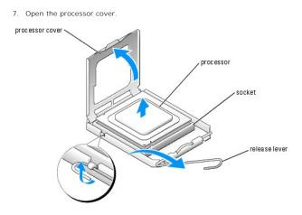
8. To remove the processor from the socket, lift the processor vertically in one motion.
